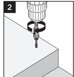
**NOTE:** Drive the screw in all at once, do not stop. You will hear a change in sound when the screw is fully driven.
